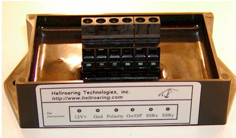
The SSR-HDVR-12P-TTLC provides for 2 control logic inputs. One for polarity logic, and one for SSR output ON or OFF. The control module requires 8 to 16 Volts for power. The outputs drive two SSR logic controls on the negative control input side. The output consists of open collector transistors which sink the SSR control input current. Internally, the control module contains circuits to prevent both outputs from being on at the same time.
