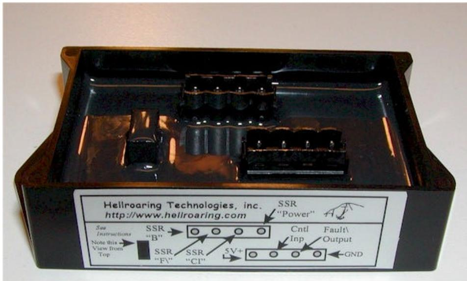
Connections should be made observing polarity! Note the orientation as viewed on the label.
